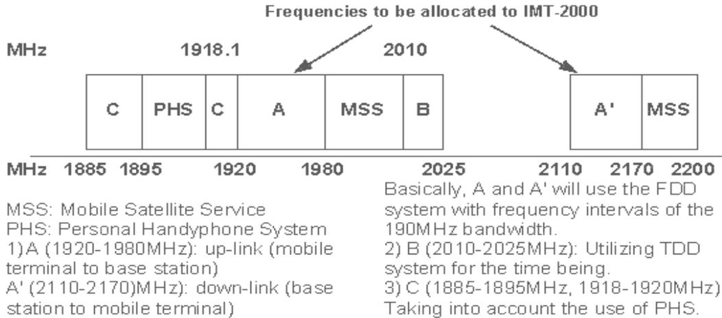
Figure 1. Frequency plan for IMT-2000.
