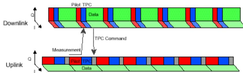
Figure 3. Multiplexing of pilot symbols.
