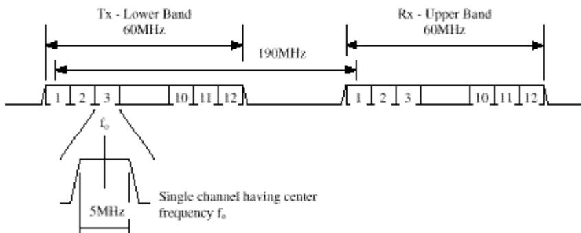
Figure 2. Operating band structure to mobile terminals.
