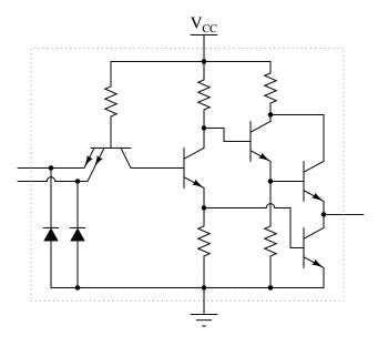
Hint: the double-emitter transistor is being used as a pair of diodes, and not as an amplifying device!
