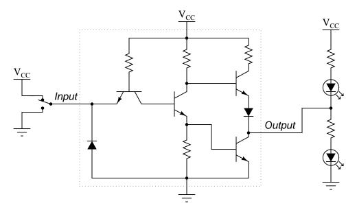
Where is the power supplied for each LED? What relationship is there between the load current (LED) and the gate input current (through the SPDT switch)?
