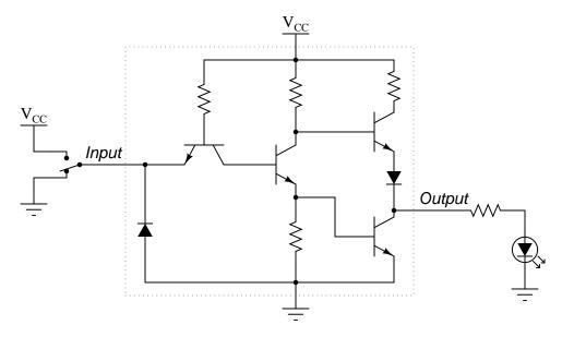
The output circuitry of this particular gate is commonly referred to as "totem-pole," because the two output transistors are stacked one above the other like figures on a totem pole. Is a gate circuit with a totem-pole output stage able to source load current, sink load current, or do both?
