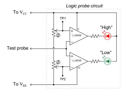
When this logic probe circuit is connected to the  $V_{CC}$  and  $V_{EE}$  power supply terminals of a powered TTL circuit, what voltage levels should test points TP1 and TP2 be adjusted to, in order for the probe to properly indicate "high" and "low" TTL logic states? Consult a datasheet for the quad NAND gate numbered either 74LS00 or 54LS00. Both are legacy TTL integrated circuits.
