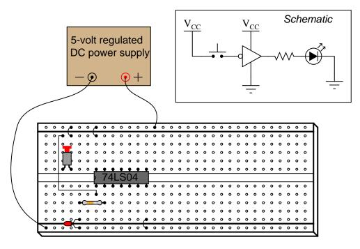
The DIP circuit is a TTL hex inverter (it contains six "inverter" or "NOT" logic gates), but only one of these gates is being used in this circuit. The student's intent was to build a logic circuit that energized the LED when the pushbutton switch was unactuated, and de-energized the LED when the switch was pressed: so that the LED indicated the reverse state of the switch itself. However, in reality the LED fails to energize no matter what state the switch is in.
