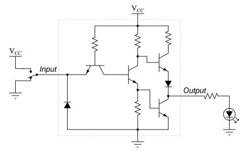
The left-most transistor in this schematic is actually not being used as a transistor, but rather it functions as a "steering diode" network, like this:
