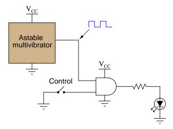
The "astable multivibrator" is nothing more than an oscillator that produces a square-wave signal at a low frequency, at standard TTL voltage levels (0 and +5 volts).
