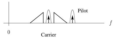
**Note:** Signals to be recovered are separated in the frequency domain (See frequency regions marked by curves)  $\Longrightarrow$  Filtering is used
