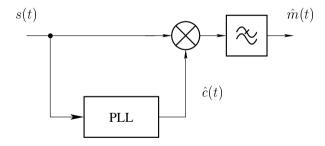
**Note:** The demodulator contains a carrier recovery circuit [its output is the recovered carrier  $\hat{c}(t)$ ] and a product detector (see the analog multiplier and low-pass filter)
