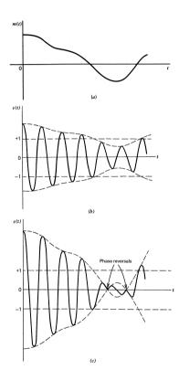
**Note:** Message signal may be recovered from the envelope only if DSB signal is a narrow-band signal  $(W << f_c)$  and if modulation factor is small enough  $(\mu < 1)$ .
