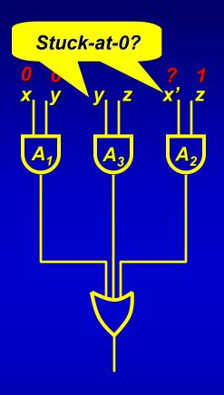
An area-optimal circuit must be fully testable for stuck-at faults.
