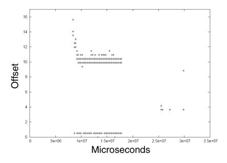
The figure above shows the results of this prediction technique for the instance described above. We can see that the two regions corresponding to the microwave interference are properly predicted and that the region of the unknown interference source is partially predicted as well. Furthermore, we see only one false positive occurring for this sample.
