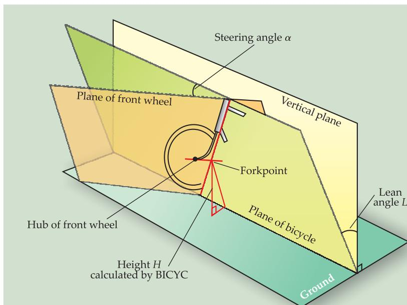
**Figure 3. A tricky trigonometrical problem.** We need to know  $H$ , the height of the forkpoint from the ground, for a leaning bicycle. Subroutine BICYC calculates both the vertical height and the height in the plane of the bike.
