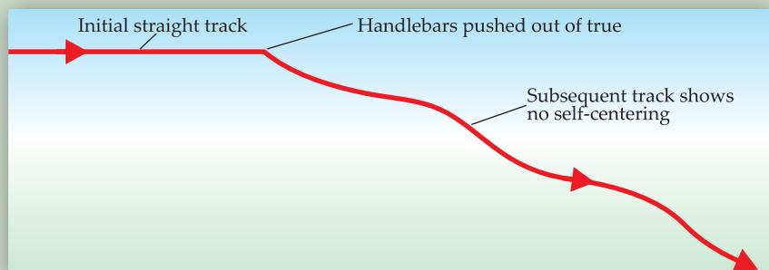
**Figure 7. Self-centering?** A bicycle with an “outrigger” third wheel to keep it upright was pushed and released riderless. At the point shown the handlebars were knocked out of true, resulting in a change of direction and no self-centering. The slight wave in the track resulted from oscillations in the framework.
