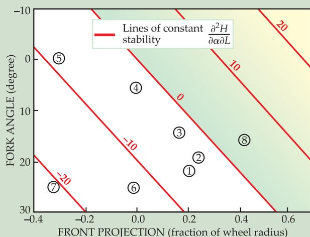
**Figure 5. Stable and unstable bicycles.** On this plot of fork angle versus front projection the  $d^2H/d\alpha dL$  lines are lines of constant stability. Shaded area shows the unstable region. Point 1 is a normal modern bicycle; 2 is a racing bike. Points 3 and 4 are high-wheelers (or “penny-farthings”) from the 1870s. Point 5 is an 1887 Rudge machine, and 6 is a Lawson “Safety” of 1879. Point 7 is URB III, and point 8, the only unstable bicycle, is of course URB IV.
