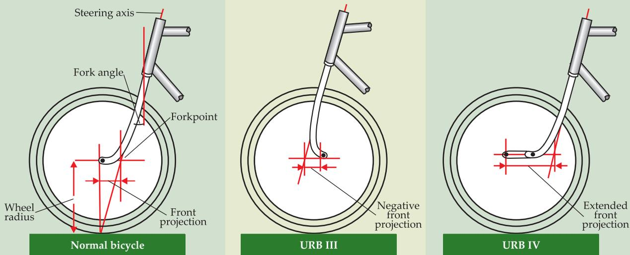
**Figure 2. Front-fork geometry.** On the left is a normal bicycle. The center shows URB III with reversed forks giving a negative front projection, and on the right is URB IV with extended front projection.
