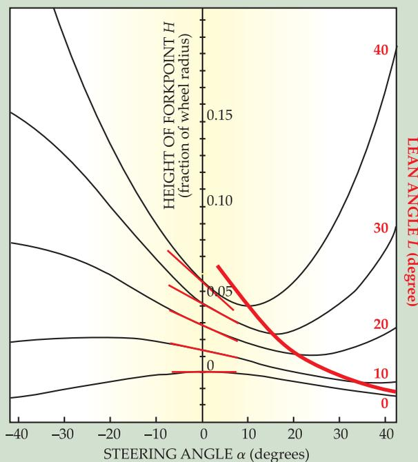
**Figure 4. Computerized bicycles.** These data, from BICYC output, show that the minimal height of the forkpoint occurs nearer to the straight-ahead position for greater angles of lean. Note also that  $dH/d\alpha$  varies linearly with lean angle  $L$  for small  $L$ . Curves, computed for typical steering geometry ( $20^\circ$  radii front projection), are vertically staggered for clarity.
