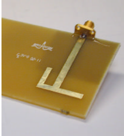
Figure 1. A printed inverted F antenna on a FR-4 substrate.
