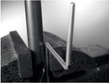
Figure 4.18: Bend the wire around the drill bit to make a coil.
