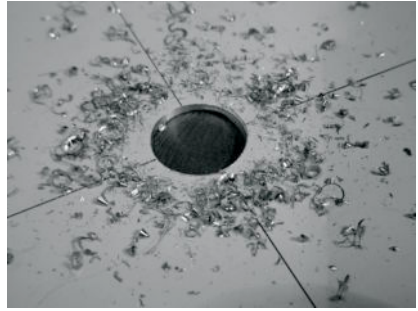
Figure 4.22: Drilling the hole in the metal plate.
