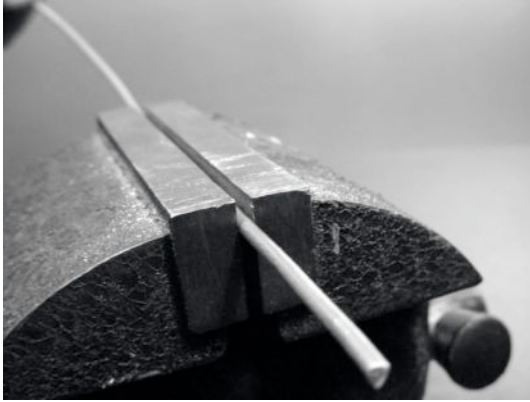
Figure 4.15: Make the wire as straight as you can.
