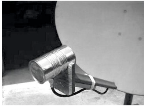
Figure 4.10: Feed horn made from a food can.
