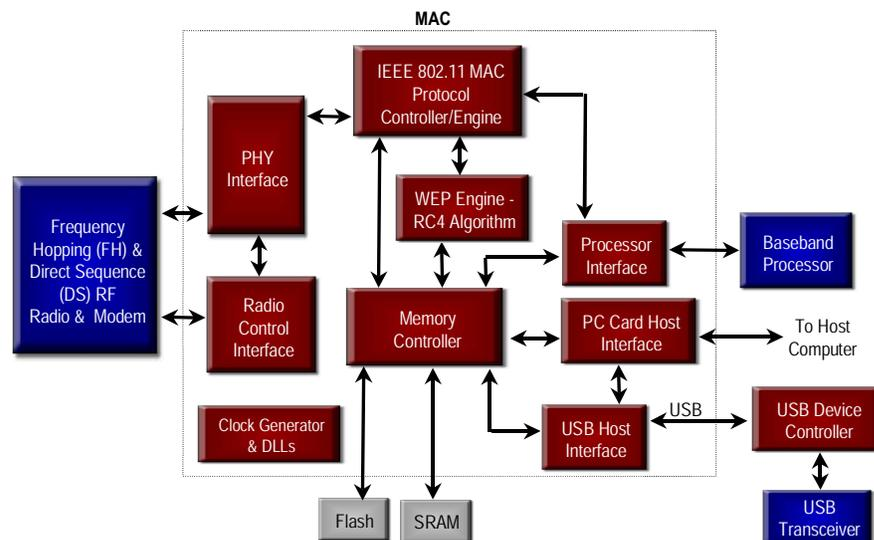
Figure 10: Wireless LAN Radio, MAC, and Baseband Controller
