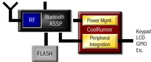
Figure 7: CoolRunner Power Management and Peripheral Integration
