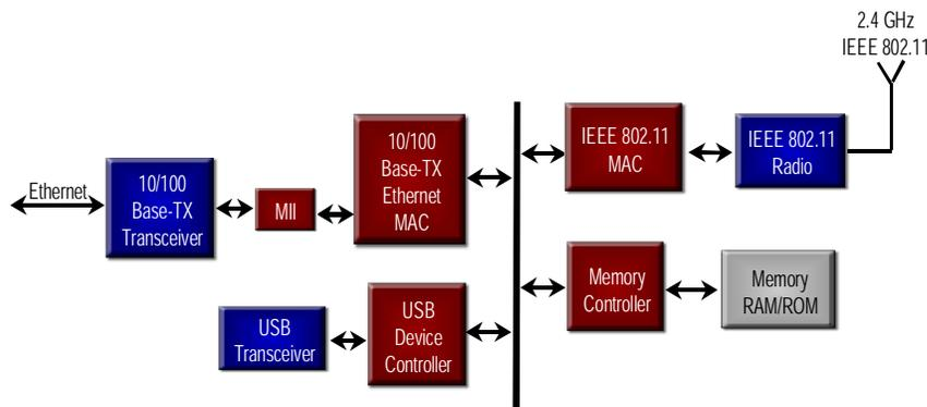
Figure 12: Spartan-II FPGAs in Wireless LAN Access Points
